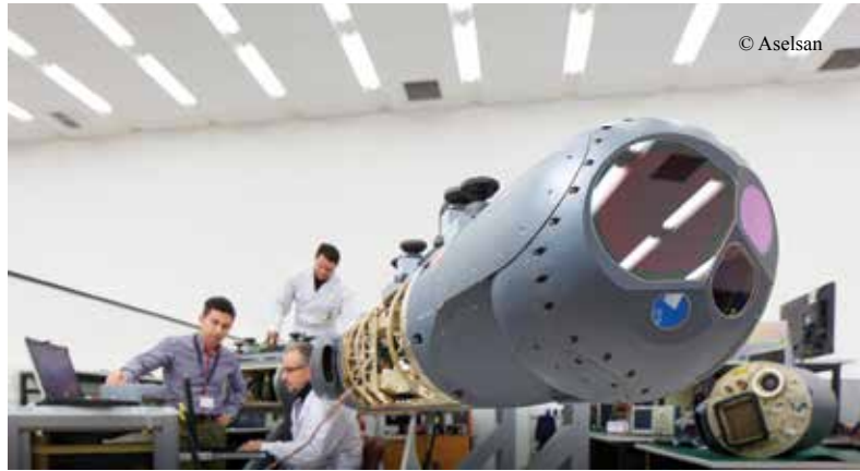
Aselpod "Advanced Targeting Pod Electro-Optical Reconnaissance, Surveillance and Targeting System"
