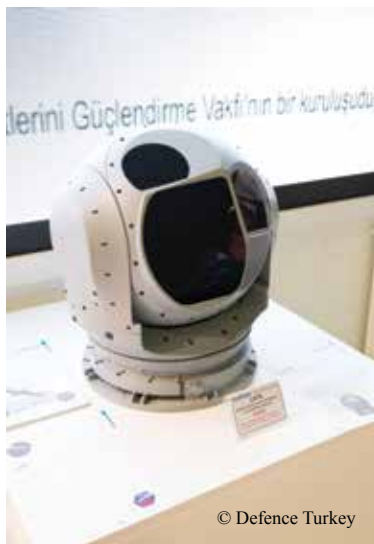
CATS - Electro-optical reconnaissance, surveillance and targeting camera
