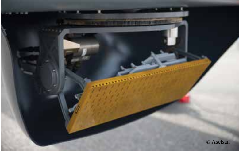
SARPER Synthetic Aperture Radar (SAR) System
