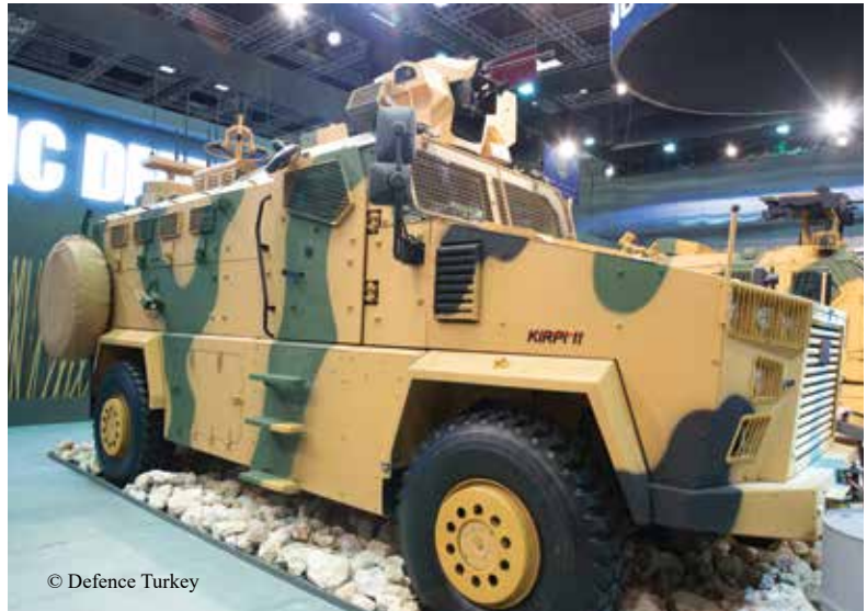
KIRPI-II New Generation MRAP was displayed at DIMDEX 2018 with Aselsan's SARP RCWS and "Yankı" Gunshot Detection System
