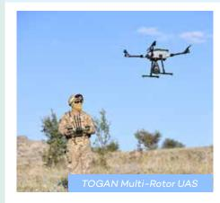
capability. A single TOGAN platform can operate for 45 minutes at a range of 10 kilometers.
