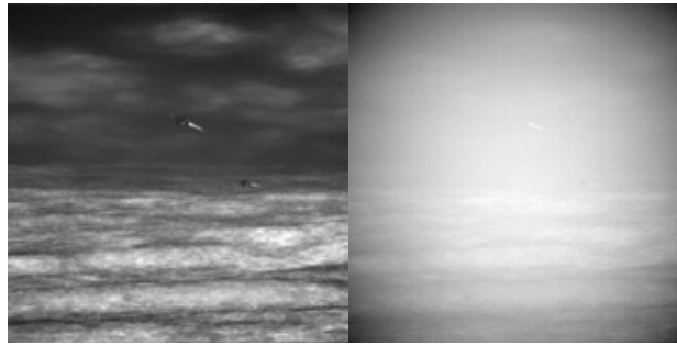
Figure-2 The effects of dome heating on the image.
