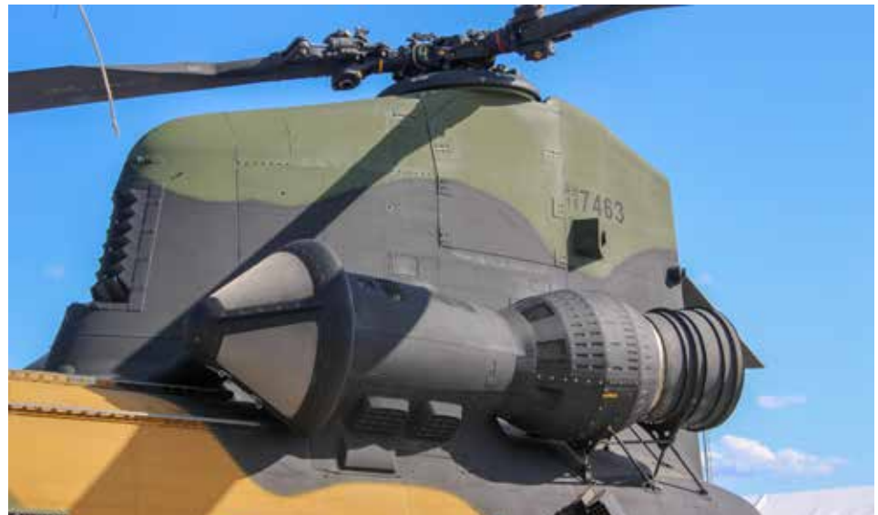
The Turkish Land Forces currently operates T55-GA-714A turboshaft engines on its CH-47F Chinook Heavy Lift Helicopters
