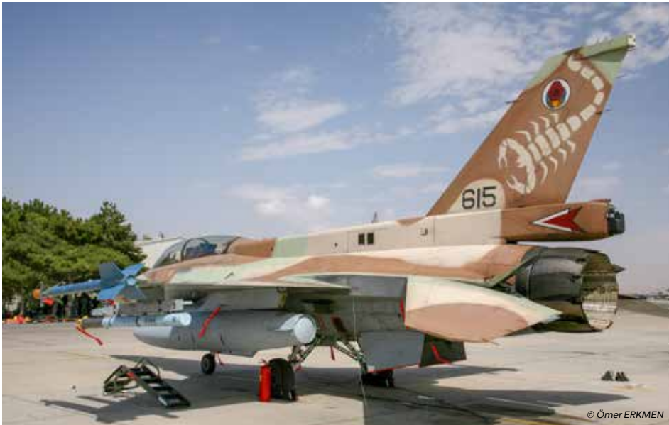
Israeli Air Force F-16D Barak aircraft is the first model to feature an ADS (Avionics Dorsal Spine). The ECM antenna is visible in the "drag chute" housing
