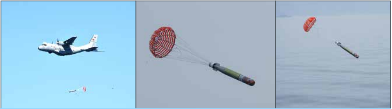
A Mk46 Mod 5A Recoverable Exercise Torpedo (REXTORP) being air launched by a Turkish Navy P235 MPA (tail number TCB653) to hunt a submarine it detected during a naval exercise. The parachute that ensures the nose hits the water first is clearly visible
