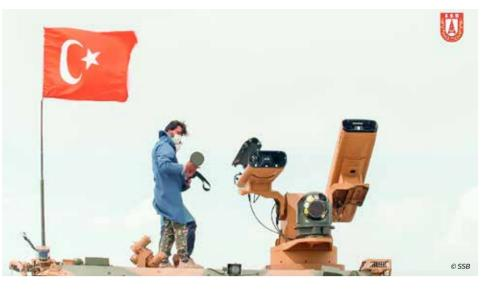
mounted atop a BMC's VURAN 4x4 Armored Vehicle. The electrically controlled turret has two PORSAV missile launcher pods, each capable of firing 2 fire-and-forget IIR guided missiles in rapid succession and is radar tracks and messages to be passed to the fire unit to alert and cue the gunner.
