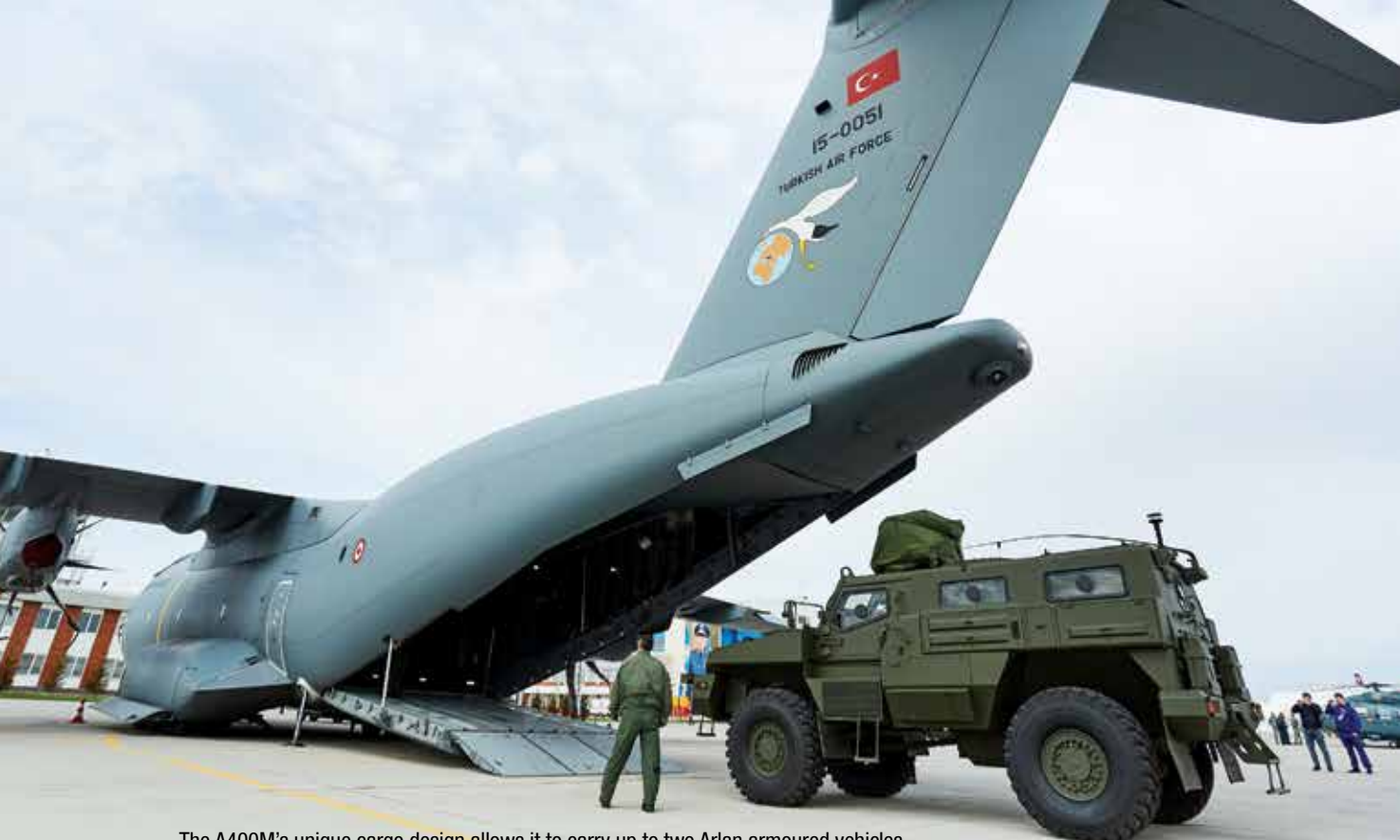
The A400M's unique cargo design allows it to carry up to two Arlan armoured vehicles, with a combat weight of 16 tons each and a height of 3.4metres
