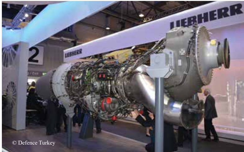
The TP400-D6 is a 3-shaft counter rotating turboprop engine delivering more than 11,600 shp
