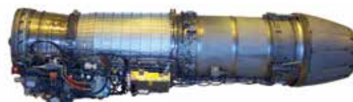
The GE's F404-GE-102 engine includes single engine safety features and a FADEC derived from F414
