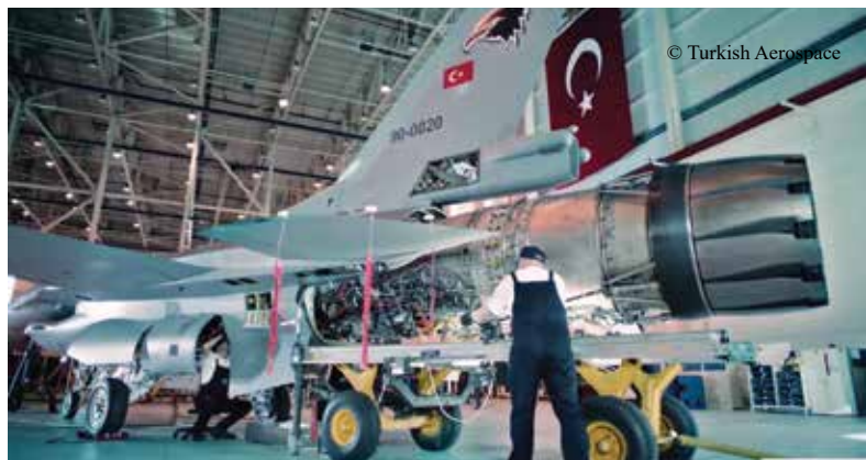
F110-GE-129 engine is seen here while being installed on a TurAF's F-16C Block 40 aircraft
