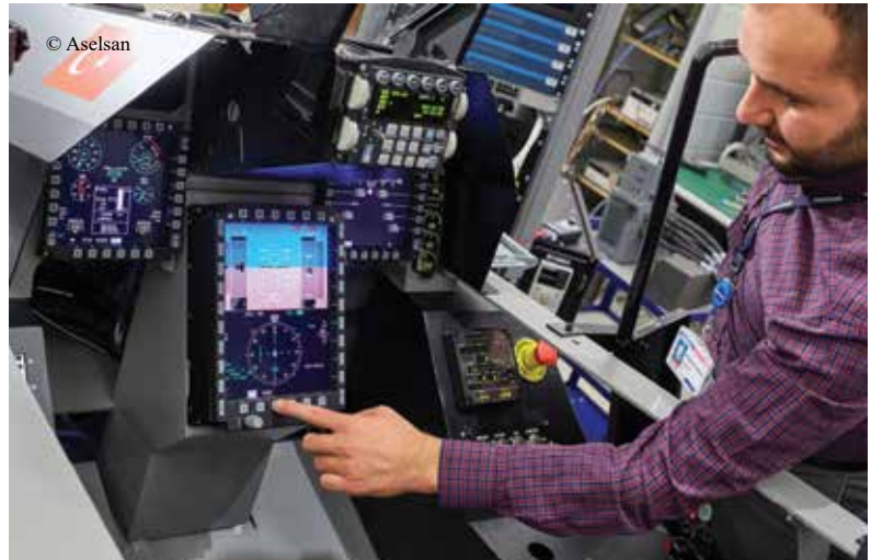
The Cockpit Demonstrator of the F-16 Block 30 aircraft developed and produced by Aselsan under ÖZGÜR Program
