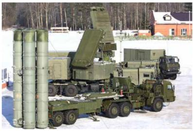
S-400 Triumph Radar Systems, 55K6E Mobile Command Systems and Launchers
