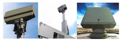
KRONOS system is to detect, track and identify targets and to provide weapons systems with targeting data, including TBM (Tactical Ballistic Missile) defence capabilities. The radars can be easily deployed, deliver high performance for a number of operational uses, and are highly reliable with graceful degradation. They are multi-functional, multimission systems, which can perform surveillance and tracking tasks both simultaneously and independently.
