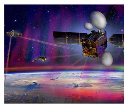
observation satellites at a distance up to 45000 km, intelligence UAVs or mission aircraft via laser. From its position in geostationary orbit, the SpaceDataHighway system relays data collected by observation satellites to Earth in near-real-time, a process that would normally around 90 minutes. It thus enables the quantity of image and video data transmitted by observation satellites to be tripled and their mission plan to be reprogrammed at any time and in just a few minutes.
