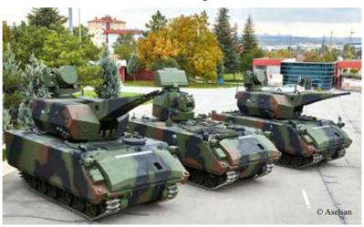
KORKUT SPAAG Vehicles are based on the FNSS ACV-30 ACV chassis
