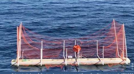
At terminal phase following sharp maneuvers at Super Sea Skimming mode ATMACA missile passed just above the radar reflector (orange object) on the fixed floating target, which represents a direct hit to the simulated target
