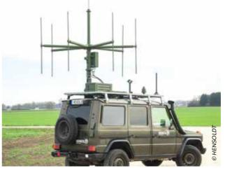
On 29 October 2019 – The passive radar "TwInvis" of sensor solution provider HENSOLDT showed outstanding detection performance during a measurement campaign of the NATO Science and Technology Organization under the leadership of the Polish armed forces.
