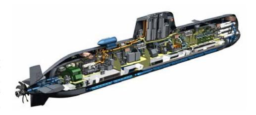
waterproof and pressureresistant submarine hull is completed. Apart from the pressure hull, the boat's construction is finalized by adding the upper deck, sail, ballast tanks (aft ballast tank is not pressurized), and the inner compartments. Because of the way the pressure hull is constructed, all the devices, systems, and equipment to be used in the submarine must be outfitted before the pressure hull blocks are combined.
