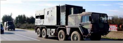
COBRA WLR of the TLFC seen here while being deployed at Turkey-Syria border
