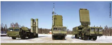
Major components of the S-400 Triumph Battery (from left to right); the 5P85TE3 Transporter Erector Launcher (TEL), X-Band 92N6E Grave Stone Engagement and Fire Control Radar and C-Band 3D 96L6E Surveillance and Tracking Radar
