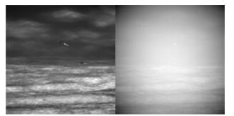
Figure-2 The effects of dome heating on the image.
