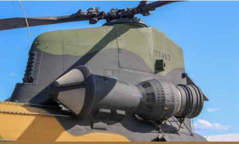
The Turkish Land Forces currently operates T55-GA-714A turboshaft engines on its CH-47F Chinook Heavy Lift Helicopters
