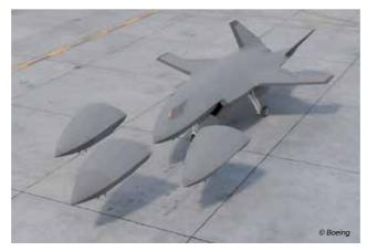
manufactured with Boeing's largest-ever resin-infused single composite piece; and assembled using proven advanced manufacturing processes.
