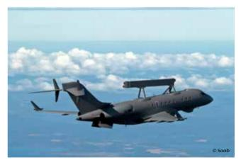
GlobalEye is Saab's new airborne early warning and control solution. It provides air, maritime and ground surveillance in a single solution. GlobalEye combines Saab's new Erieye Extended Range Radar and a range of additional advanced sensors with the ultralong range Global 6000 aircraft from Bombardier.
