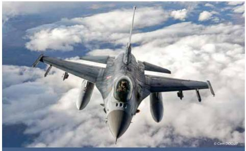
Turkish Air Force F-16C Block 50M aircraft were equipped with the AN/ALQ-178(V)5+ ECM system under the SPEWS-II project. The distinctive ECM antennas are an integral part of the formation lights
