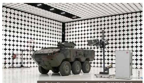
Otokar Electromagnetic Compatibility (EMC/EMI) Test Center
