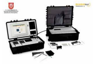
The system has become capable of detecting ELISA and PCR reactions simultaneously and also in the field.
