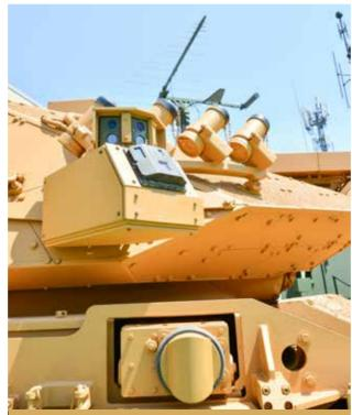
From top to the bottom YAMGOZ Close-Range Surveillance System sensor, Tank Laser Warning Receiver System (TLUS) sensor and AKKOR PULAT APS Counter Measure Module
