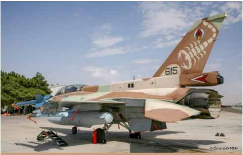
sraeli Air Force F-16D Barak aircraft is the first model to feature an ADS (Avionics Dorsal Spine). The ECM antenna is visible in the "draa chute" housina
