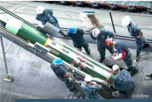
A Mk48 HWT being loaded into a US Navy submarine
