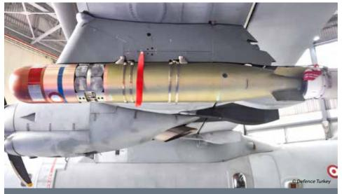
P235 MPA of the Turkish Navy can be armed with two lightweight-to-pedoes for the Anti-Submarine Warfare (ASW) role. An Mk46 Mod 5A REXTORP seen here at P235's underwing pylon.
