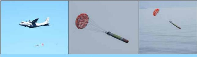
A Mk46 Mod 5A Recoverable Exercise Torpedo (REXTORP) being air launched by a Turkish Navy P235 MPA (tail number TCB653) to hunt a submarine it detected during a naval exercise. The parachute that ensures the nose hits the water first is clearly visible
