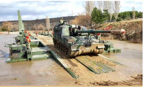
T-155 Self-Propelled FIRTINA Howitzer is seen crossing over the river thanks to the OTTER -Rapid Deployaple Amphibious Wet Gap Crossing System
