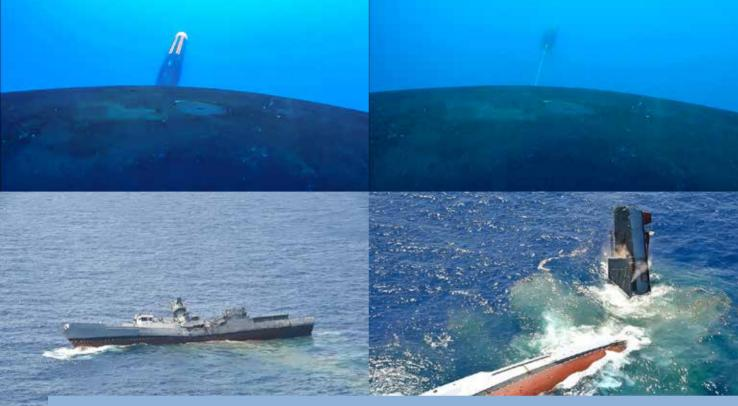
During the White Storm 2016 Exercise, which also included a live-fire ship sinking mission, a decommissioned Tepe (Ex US Navy Knox) Class Zafer Frigate was used for target practice. The lethal effect of the DM2A4 HWT that was launched by a GUR Class Submarine on the Zafer Frigate highlighted in sequences. The DM2A4 HWT hit the Zafer amidships, breaking her keel and sending her below.
