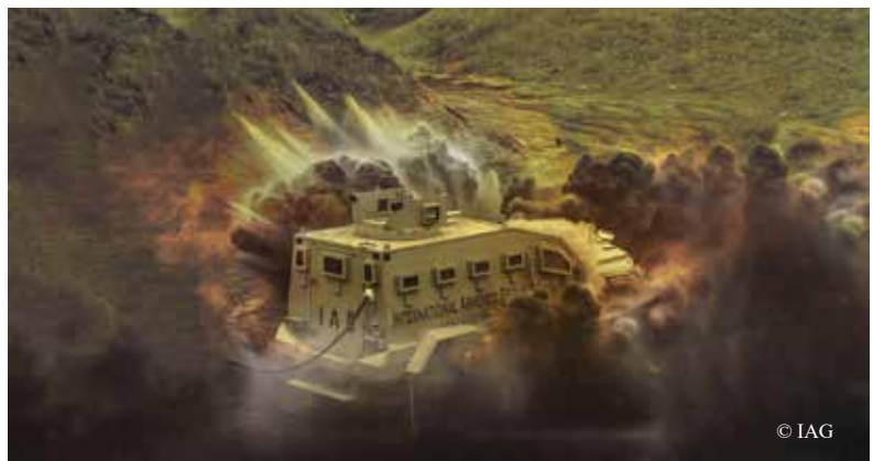
The footage of IAG Guardian Xtreme MRAP -STANAG-4569 Level 3a mine/blast test
