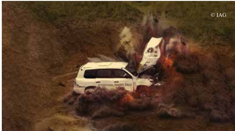
The footage of VPAM BRV 2009 VR7 certified Toyota Land Cruiser 200 series vehicle - the Stanag 4569AEP55 Level 2a mine test
