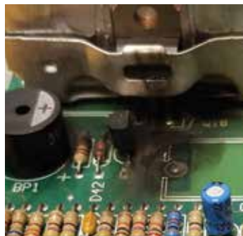
Figure 6: Blown transistor caused by generator frequency deviation
