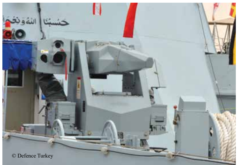
Aselsan's 25mm STOP Remote Controlled Stabilized Naval Gun System seen here onboard PN's Himmat Fast Attack Craft anchored at NAVDEX Pontoon
